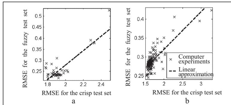
Fig. 8. Comparison of discrepancies obtained for fuzzy and crisp test sets after model tuning using a fuzzy training set for the Mamdani model (a) and Sugeno model (b).
