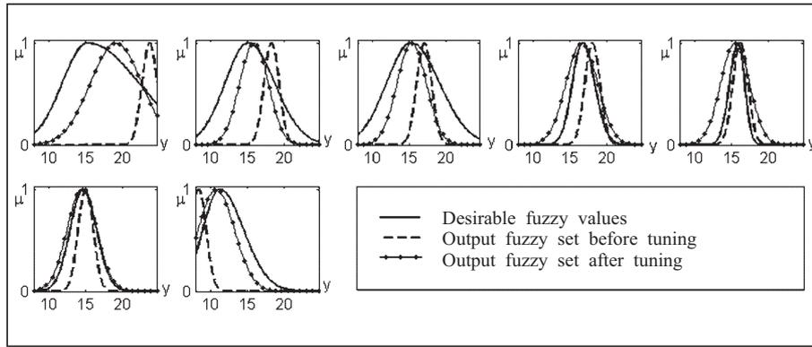
Fig. 6. Fuzzy output values of the Sugeno model for the test set.
