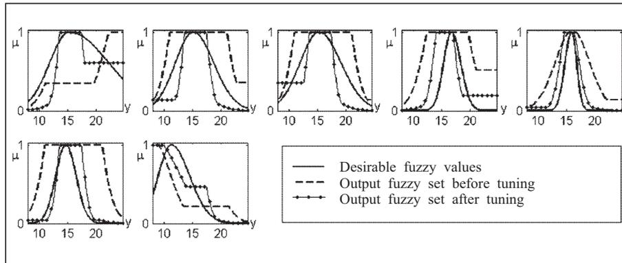
Fig. 5. Fuzzy output values of the formed Mamdani model for the test set.
